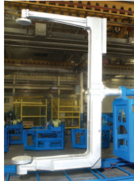
"C" Style Offset Arm; the "C" support is removable
