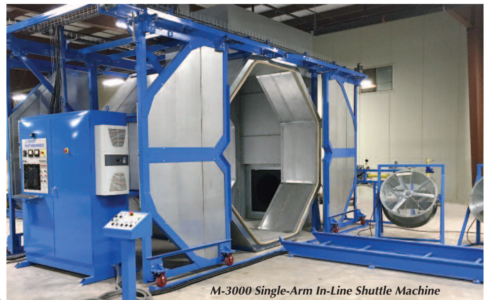
In-Line Shuttle machines provide a single oven and one or two arm/carts: 1. Oven, 2. Arm/Cart, 3. Additional Arm/Cart Cooling, Unloading & Loading all occur in the station outside the oven.
