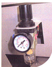
Integrated air control assembly
